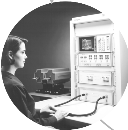
85106D with option 001, 45 MHz to 50 GHz in coax, above 50 GHz in waveguide
